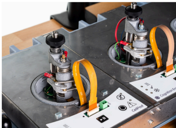
Figure 15: Cell loaded into CellPod with temperature gradient sensor strip correctly installed
