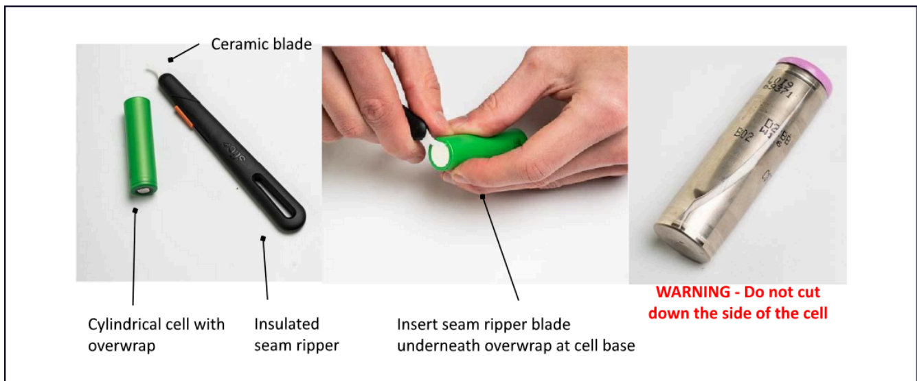
Figure 13: How to strip a cell of its plastic wrapper correctly
